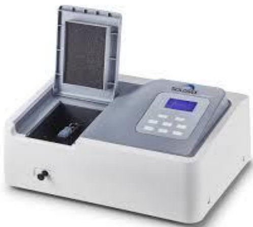
A spectrophotometer. Image credit: SCIOLOGEX
